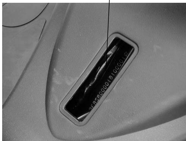
Location of Frame Serial Number
