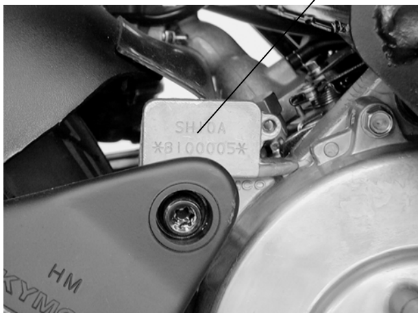
Location of Engine Serial Number
